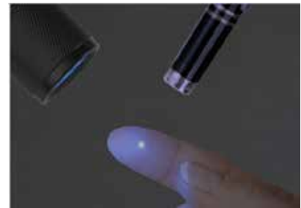
A single Microtaggant Identification Particle with upconverting phosphors, illuminated by an infrared laser pen.
